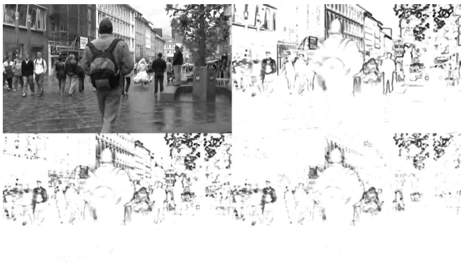
Fig. 2. Stillshot from a video (top left quadrant) and the corresponding geometrical invariants. For invariant K (bottom right quadrant), non-white locations change in all three spatio-temporal directions, whereas for S (bottom left), the video signal changes in at least two directions. Additionally, invariant H (top right) also responds to stationary edges and uniform regions that change in time (i.e. one dimensional changes). The (small) response even of K at the corners of the windows is due to small camera vibrations and noise. For the invariants, the brightness has been thresholded and inverted for better legibility.
