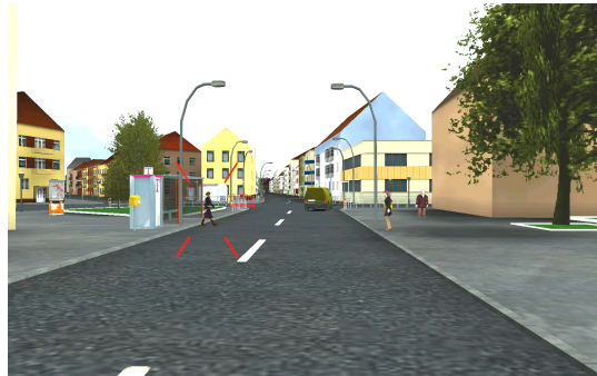
Fig. 1: Simulator scene. Because the driver is looking away, the pedestrian beginning to cross the street is highlighted with a gaze-contingent cue.
