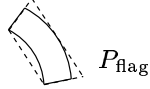
Fig. 1. Sector defined by an orientation and distance interval reconstructed by inverse quantization of raw server data representing the possible true relative positions of a landmark flag w.r.t. the agent. The solid line represents the form of the area as derived by the raw data. For the polygon algorithms, the area is slightly enlarged to the polygon denoted by the dashed lines.
