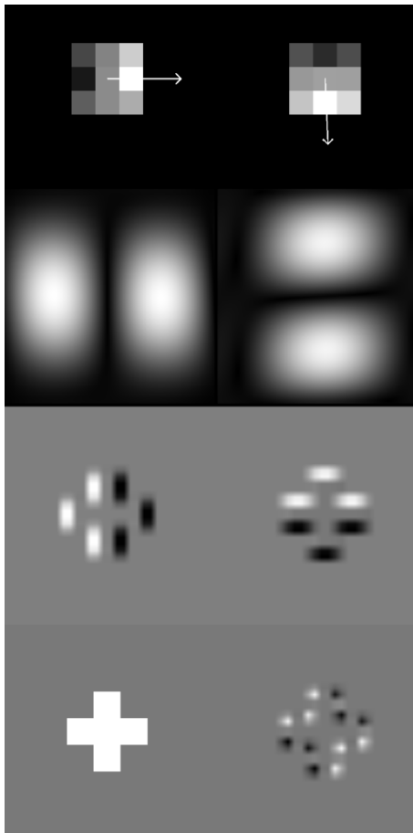
Figure 12. An example of learned filters pairs. The top row shows the two learned 3 \times 3 filters (arrows indicate orientation) and the row below the corresponding Fourier spectra. The third row depicts the responses of the two filters to the image shown in the bottom left (image used as T_1 to illustrate the selectivity of the FP-unit). The bottom-right panel shows the response of the FP-unit (the product of the filter responses). Such textbook units, however, are rather rare. This particular unit has emerged in the FP-net-59 trained on Cifar-10 without instance normalization and without the ReLU in Equation 2.
