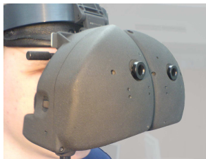
Fig. 2. Picture of our head-mounted display. Note the two scene cameras facing forward; two gaze cameras are integrated into the case.
