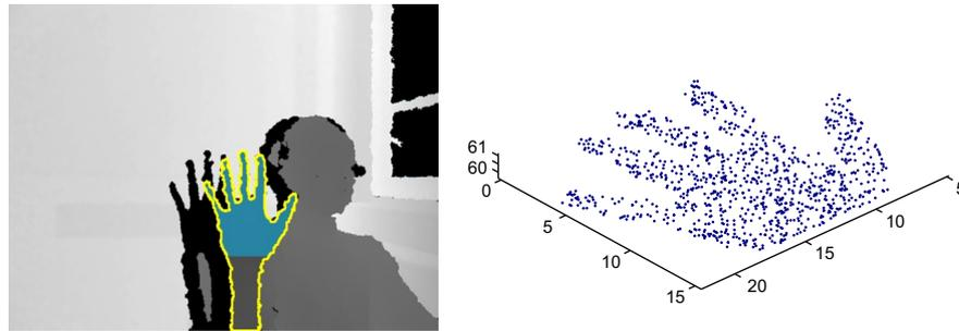
**Fig. 6.** Starting from a frame captured with the Kinect, we extract the hand based on the closest object assumption. We remove the points corresponding to the forearm and obtain the segmented hand and the 3D point cloud used for the tracker's learning stage.
