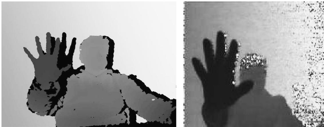
Fig. 10. Depth stream comparison: Microsoft Kinect (left) and PMD CamBoard Micro (right).
