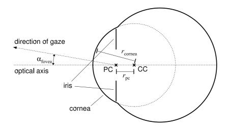
Figure 2. Eye model used in the remote gaze estimation algorithm. PC: Pupil centre. CC: Cornea centre.  $r_{cornea}$ ,  $r_{pc}$ ,  $\alpha_{fovea}$ : User-dependent parameters (see text for explanation).
