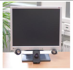
Figure 1. Remote eye tracker system setup. The eye tracking hardware consists of a single high-resolution camera below the display and two infrared LEDs to either side.
