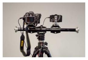
The no parallax requirement implies that the second camera must take the position of the first when shooting. A practical solution offering high precision is shown in Figure 3. By rotating the accessory arm by 180 degrees one camera can take the position of the other. In the case of ideal camera adjustment the entry pupils of both cameras are matched by the rotation.
