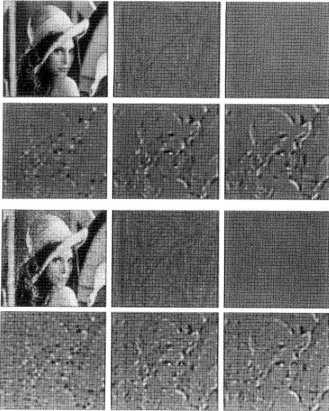
FIG. 2.1. Traditional geometric measures H and K compared to the more robust clipped eigenvalues (defined in Eq. 16). Results are illustrated as gray-level images with “gray” for zero, “bright” for positive, and “dark” for negative values of the corresponding measures. First row: mean (in the middle) and Gaussian curvature (on the right) of the natural intensity surface shown on the left. Second, row: output of the clipped eigenvalues operator (Eq. (16)) for n = 2, 4, 6 (from left to right) and A(\rho) = (2\pi\rho)^2 \exp(-\pi\rho^2/4\sigma_f^2) including a Gaussian blurring with a space constant \sigma = 1.8 pixels ( \sigma = 1/4\sigma_f ). The same operations are repeated below for a noisy input (25% uniformly distributed additive noise).
