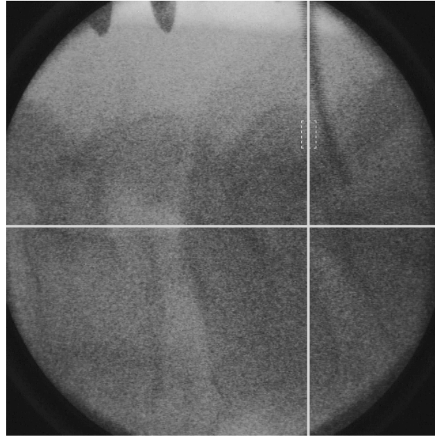
Figure 3. Fluoroscopy sequence frame with simulated defective lines and columns. For better visibility, the defects are represented with maximum gray level. The rectangle indicates a region for which enlarged results are shown later on.
