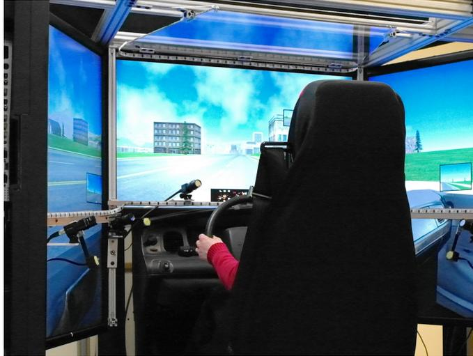
Figure 1: View of the state-of-the-art FAAC driving simulator. The system emulates the interior of a car, in which the windshield, covering a horizontal field of view of 225 degrees, is simulated using five LCD panels. The simulator is integrated with a six-camera Smart Eye PRO eye tracking system. The gaze-contingent warnings are implemented using LED arrays mounted horizontally; the LED arrays can be seen above the central monitor and on the horizontal bar slightly above steering wheel height.
