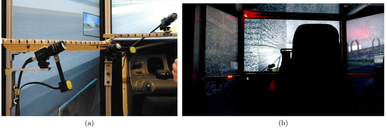
Figure 2: Left: LED strip mounted on aluminium profiles across the bottom edge of the simulated windshield. Right: Stillshot of a gaze-contingent cue to the left during a data recording session. The subject was driving in an urban environment, in combined night and rain conditions. The cue started in the centre of the LED arrays and then rapidly moved leftward to capture the driver’s attention.
