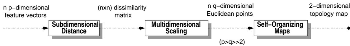
**Figure 1.1: Data flow through mapping infrastructure.**
