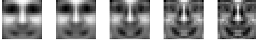
Fig. 2. Face detection templates. From left to right the average face ( \alpha = 1 ) and the subgaussian templates are shown for \alpha = 10, 20, 100 and \alpha \rightarrow \infty .
