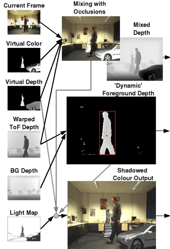
**Figure 9:** Overview of the color mixing and shadow casting of real and virtual objects on the GPU. On the left hand side, all the input images are displayed. Based on the different depth images, mutual occlusions can be handled in the augmentation. Moreover, foreground-segmented depth images and mixed depth images are delivered. The scaling of the augmented image via the light map yields the final color image output (from [SBK\*08a]).
