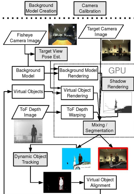
**Figure 7:** System for 3D environment modeling, 3D object tracking and segmentation for Mixed Reality applications (from [BSBK08]).
