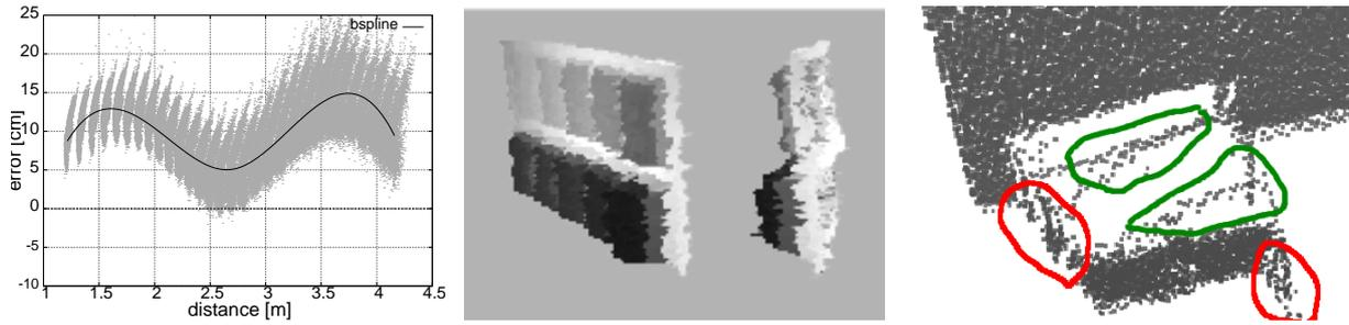
**Figure 3:** Error sources of PMD-based ToF cameras. Left: Systematic distance error for all pixels (grey) and fitted mean deviation (black). Middle: Intensity-related distance error when sensing a planar object with varying reflectivity. Right: Motion artifacts (red) and flying pixels (green) for a horizontally moving planar object in front of a wall.
