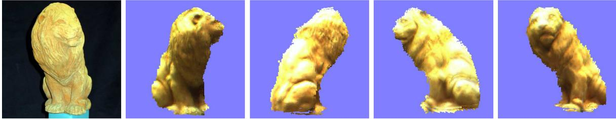
**Figure 12:** RGBz light field example from [TRSKK08], where a PMD Vision 19k camera was used. The artifacts result from the inaccurate depth information at the object boundaries.
