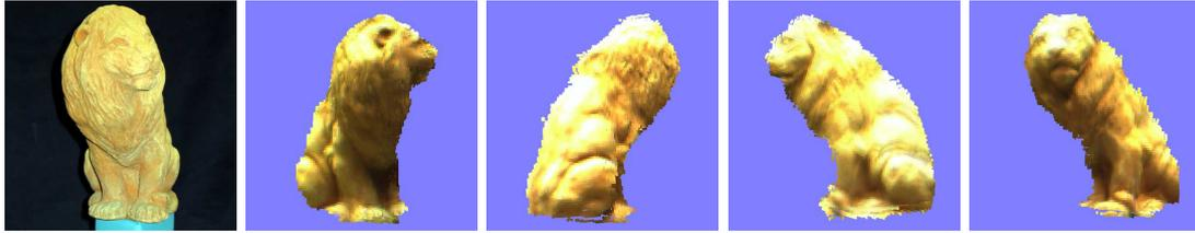
**Figure 12:** RGBz light-field example from [TRSKK08] using a ToF-sensor. A PMD Vision 19k camera has been used. The artifacts result from the inaccurate depth information at the object boundaries.
