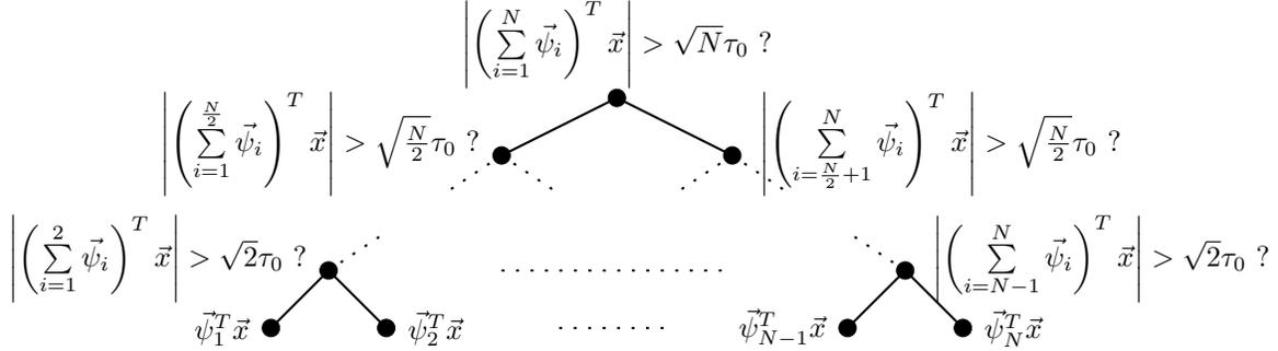
Figure 1: Schematic illustration of an AHS tree. During sensing, AHS partially traverses the tree. For each visited node, one measurement, i.e., the inner product of the unknown signal  $\vec{x}$  with a particular measurement vector, is conducted.
