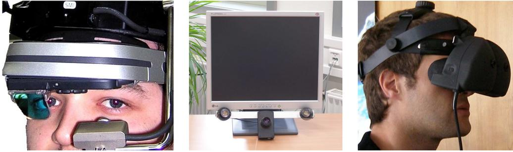
**Figure 1.** Hardware currently used to incorporate eye tracking technology into visual communication systems. Left: Monocular head-mounted display worn together with a head-mounted EyeLink eye tracker. Middle: Remote eye tracker attached to a standard TFT screen. Right: Custom-built head-mounted display with integrated binocular eye tracking and two outward-facing scene cameras.
